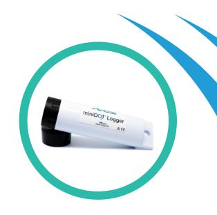
The miniDOT<sup>®</sup> Logger is a completely submersible instrument that logs dissolved oxygen and temperature measurements. The oxygen sensor is an optode that measures dissolved oxygen concentration in water through a fluorescence method. Data are recorded to an internal SD card. Operation of the miniDOT logger such as setting the time and sample interval can be accomplished via the USB cable.
