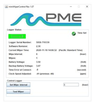
The miniWIPER must be connected to USB at this time. When correctly connected the miniWIPER LED will display a constant green light.
