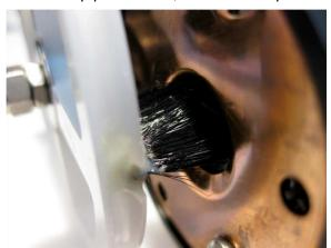
bristles to "pole vault" while in contact with the foil. Hopefully, this action will be detrimental to whatever fouling organisms are attempting to colonize the foil.
