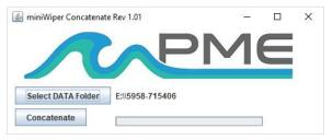
The miniWIPERConcatenate program reads and concatenates the files recorded by the miniWIPER. This program produces a CAT.txt file in the same folder as selected for the data. The CAT.txt file contains all the original measurements and contains two additional statements of time.
