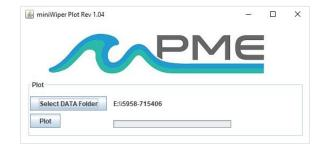
all the miniWIPER files in a folder, except the CAT.txt file. Select the folder that contains the files recorded by the miniWIPER. If the miniWIPERPlot program is run directly from the miniWIPER, then the program will suggest the folder that is located on the miniWIPER's SD card. You may accept this by clicking "Plot", or you may click "Select DATA Folder" to browse to your HOST computer's hard
