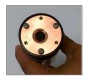
While maintaining the alignment (pictured right), slide miniWIPER and miniDOT Logger relative to each other until the brush engages the sensing foil as shown below. You may rotate the small pulley slowly by hand. This causes the internal motor to turn but will not damage miniWIPER.
