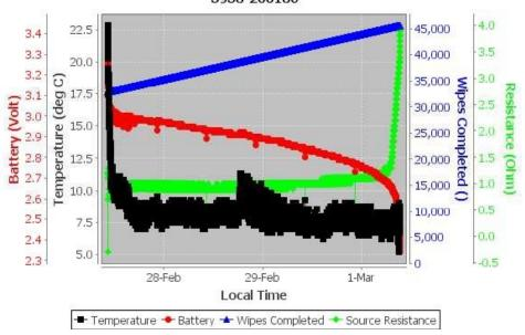
Energizer L91 Lithium AA at 4 deg C. 12785 single scrub wipes, no pressure.
