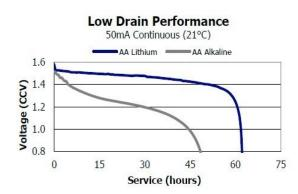
safety factor of 2 for shallow water and 4 for deep water when planning battery life.
