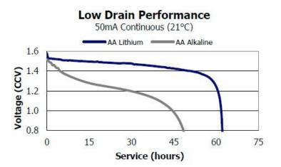
The figure (left) gives a general idea of terminal voltage vs. lifetime. Service life in hours is incorrect since miniWIPER draws 50 to 100 mA depending on various factors, but the general shape of the voltage vs. time gives an estimate of life remaining. This plot is taken from the manufacturer's specification. The plot is for a single battery. The miniWIPER halts operation at a total of 2.8 Volts.
