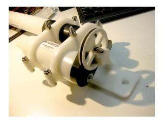
Rotate miniWIPER and Cyclops 7 Logger until the Cyclops 7 Logger optical surface and the wiper pulley axes are as shown in the pictures.
