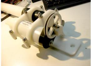
Your miniWIPER will provide a gentle brush action across the Cyclops 7 optical surface, which is intended to reduce or eliminate fouling organisms. This wiper is an accessory for the Cyclops 7 that can be added at any time.
