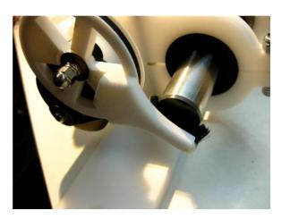
Tighten the 6 bolts while maintaining the miniWIPER and Cyclops 7 positions. First tighten the 4 outer bolts until the gap in white plastic closes. Next tighten the inner two until the miniWIPER and Cyclops 7 Logger are securely held. A small gap in white plastic on these inner bolts will remain when all is secure.
