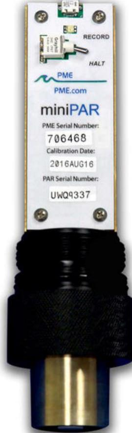
2. Move the Logger Control Switch to the “Record” position. The LED will flash green 5 times. The miniPAR Logger will now record a measurement of time, battery voltage, temperature, PAR, and 3 axis acceleration every 10 minutes (or at some other interval you may have set using the miniPARControl program). The logger will start recording measurements at the start of the next minute.
