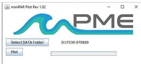
The miniPARPlot program plots the files recorded by the miniPAR Logger. The program reads all the miniPAR Logger files in a folder, except the CAT.txt file. Select the folder that contains the files recorded by the miniPAR Logger. If the miniPARPlot program is run directly from the miniPAR Logger, then the program will suggest the folder that is located on the miniPAR Logger’s SD card.
