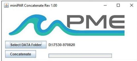
The miniPARConcatenate program reads and concatenates the files recorded by the miniPAR Logger. This program produces a CAT.txt file in the same folder as selected for the data. The CAT.txt file contains all the original measurements and contains two additional statements of time. CAT.txt is CSV (comma-separated values) file and can easily be imported into Excel and other
