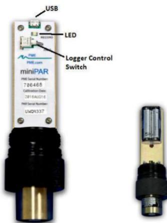
Removal of the cover reveals the miniPAR Logger’s connections and controls, shown here.
