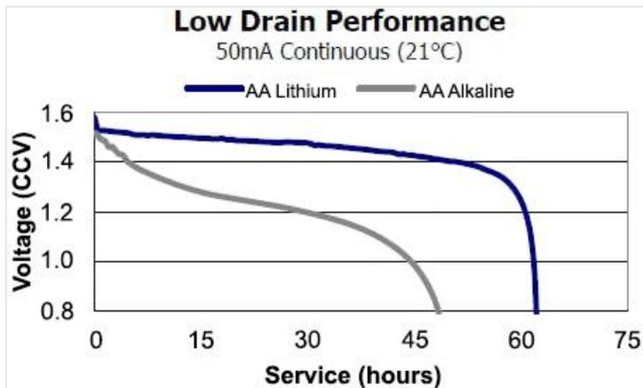
The figure below gives a general idea of terminal voltage vs. lifetime. Service life in hours is incorrect since miniPAR Logger draws far less than 50 mA continuously, but the general shape of the voltage vs. time gives an estimate of life remaining. This plot is taken from the manufacturer's specification. The plot is for a single battery. Double the voltages shown to give the terminal voltage as measured in the picture above. The miniPAR Logger halts operation at a total of 2.4 Volts.
