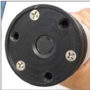
2. Position the Copper Plate faced down so that the notches in the Copper Plate perfectly align over sensing foil and over the screw holes.
