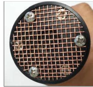
*CAUTION: Environments where debris can get trapped inside the sensing area should be avoided when using this product. PME recommends using the Cu plate in such environments.*
