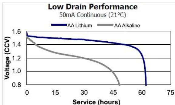
The figure below gives a general idea of terminal voltage vs. lifetime. Service life in hours is incorrect since miniDOT Logger draws far less than 50 mA continuously, but the general shape of the voltage vs. time gives an estimate of life remaining. This plot is taken from the manufacturer's specification. The plot is for a single battery. Double the voltages shown to give the terminal voltage as measured in the picture above. The miniDOT Logger halts operation at a total of 2.4 Volts.
