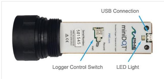
The **LED Light** is a LED that can display either red or green light. This is used to indicate the different features described in Chapter 1 in this manual.
