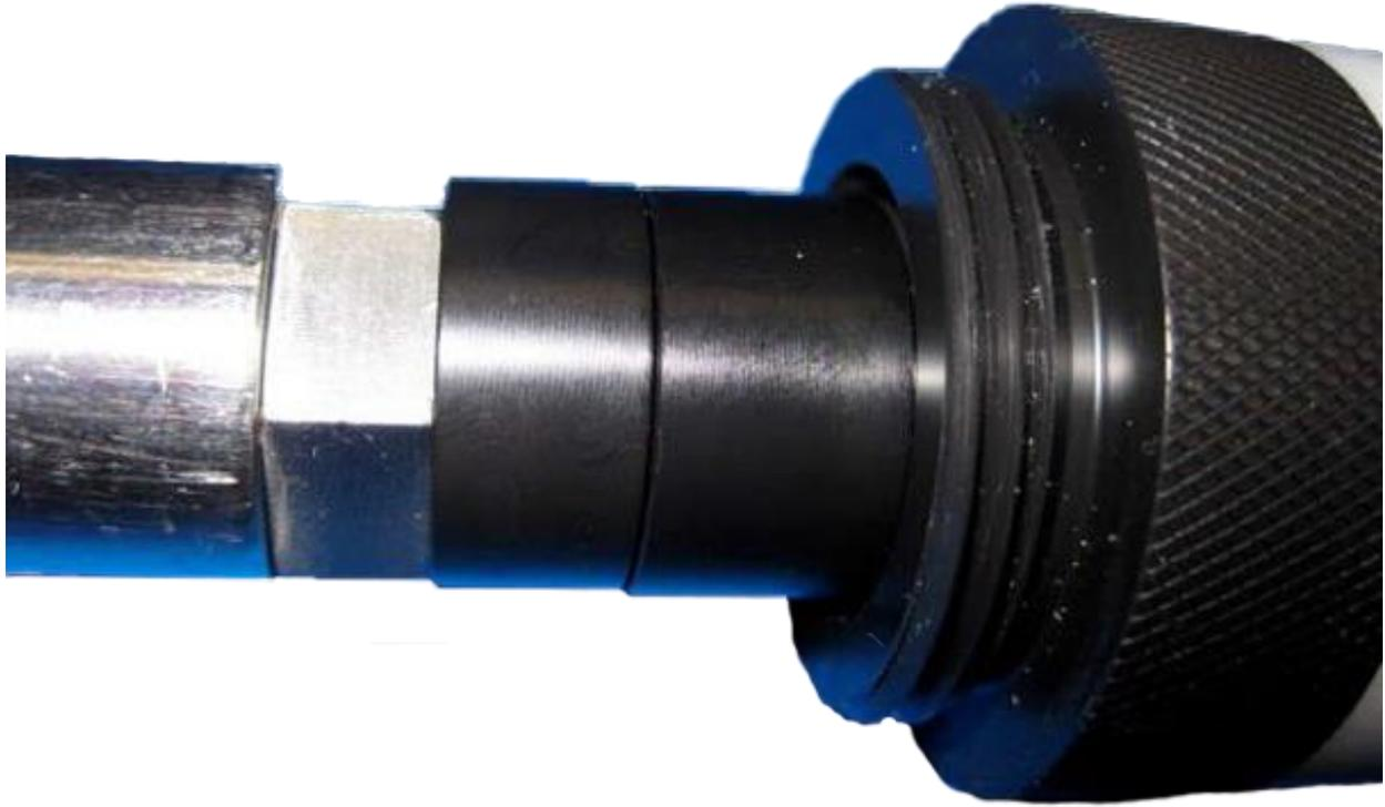
Slide the sensor support (middle-right in first picture) over the sensor. Note this part has an internal o-ring that comes against the sensor. This is not a water-proof seal. Its purpose is to firmly secure the sensor within the support. Next screw the sensor guard (middle left in first picture) onto the sensor support. The completed assembly is shown in the picture below.
