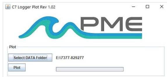
C7Plot plots the files recorded by the Cyclops-7 Logger. The software reads all Logger files in a folder, except the CAT.txt file. Notice that the software has automatically suggested the Cyclops-7 Logger SD card as the Data Folder. You may accept this or click Select DATA Folder to find some other source for the plot.
