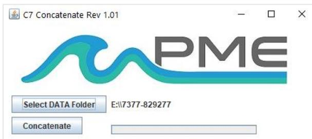
Cyc7Concatenate concatenates the files recorded by the Cyclops-7 Logger. The software reads all Logger files in a folder, except the CAT.txt file. Software translates Logger time stamps into two additional formats and saves the result in a CAT.txt file in the DATA Folder.
