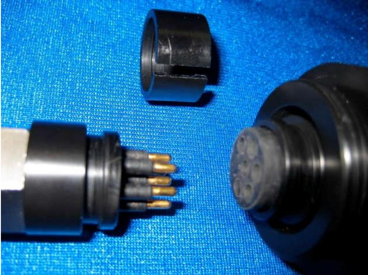
Be sure both are fully screwed on. If either is not, the clip will hold the sensor in a position where it may not make full contact with the connector.
