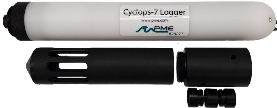
The small circular black clip shown to the right of the C7 sensor will be found installed on the logger connector. This can be removed by unscrewing it from the connector, and then gently prying open the 'C' clip center piece.
