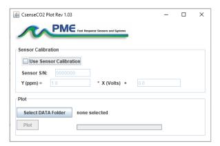
CsenseCO2Plot plots the files recorded by the C-sense Logger. The software reads all C-sense files in a folder, except the CAT.txt file. The software will also compute CO2 saturation from the voltage measured of the sensor. To do this software must be given the sensor calibration. The sensor manufacturer supplies the sensor calibration. If the Use Sensor Calibration is checked the plot will display calibrated values. If not checked the plot will display sensor output in Volts.
