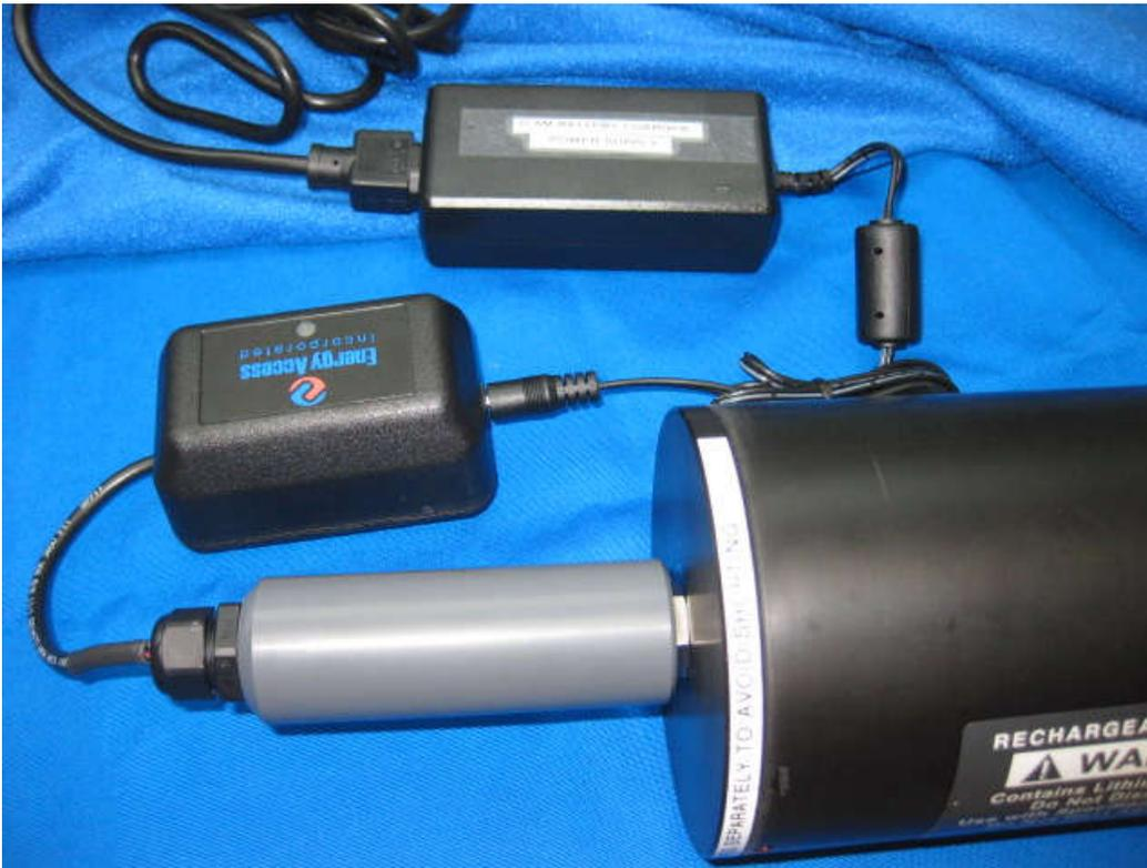
Connect the battery charger. The charger will require power from a power supply. The charger has a LED light indicating the status of the charging.
