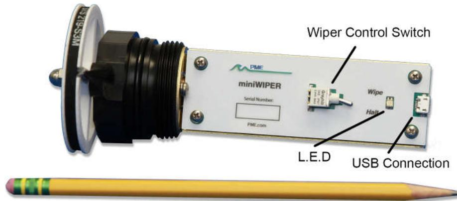
The **LED Light** is a red or green LED. This is used to indicate different features described elsewhere in this manual.
