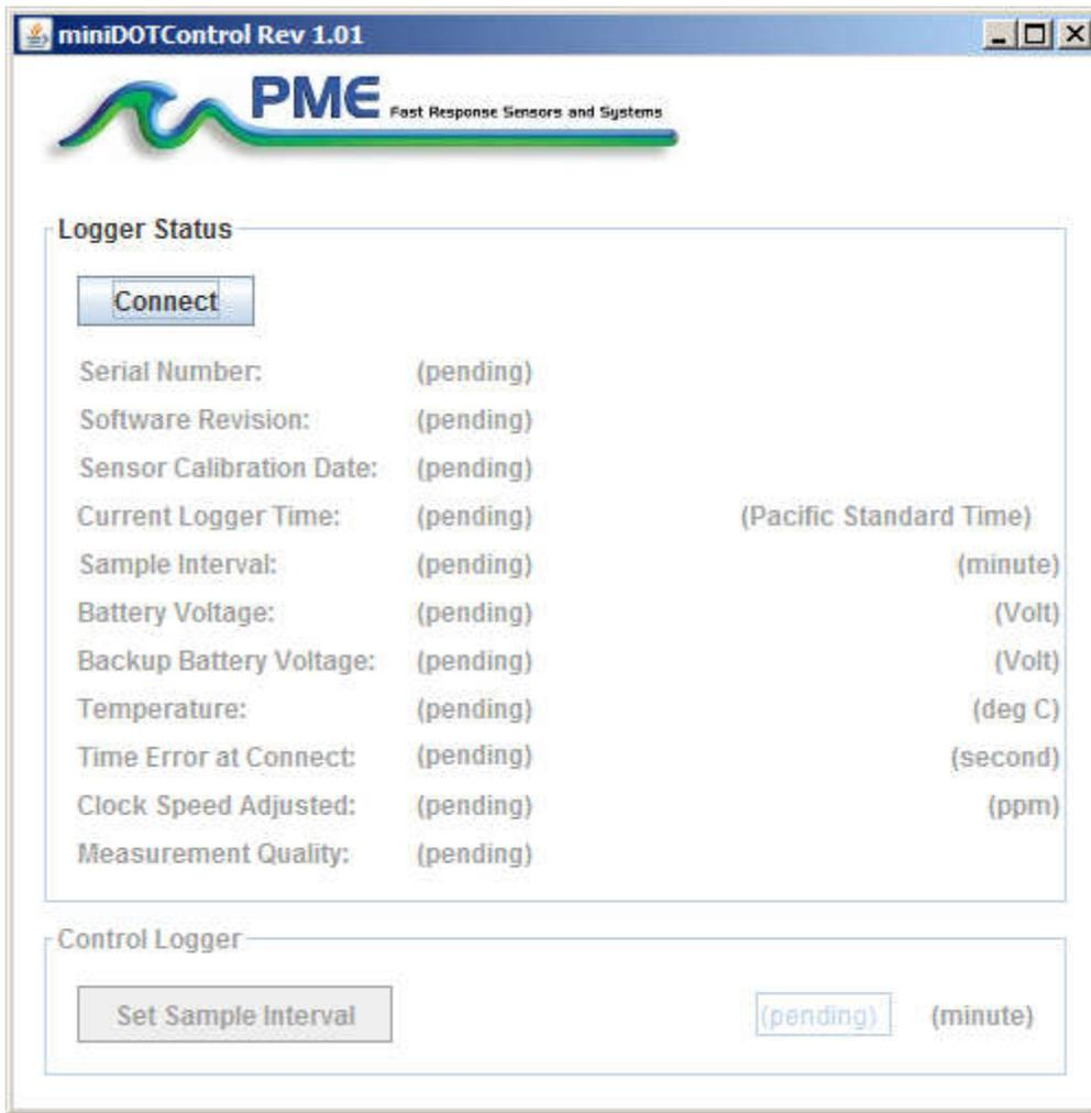
The miniDOT Logger must be connected to the HOST computer via the USB connection at this time. When correctly connected, the miniDOT Logger's LED will display a constant green light.
