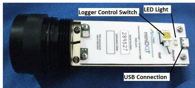
The **LED Light** is a LED that can display either red or green light. This is used to indicate the different features described in Chapter 1 in this manual.
