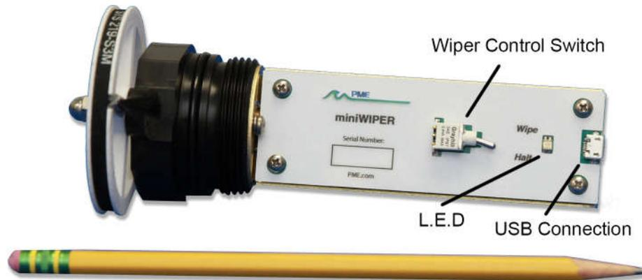
The **LED Light** is a red or green LED. This is used to indicate different features described elsewhere in this manual.
