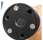
2. Position the Copper Plate faced down so that the notches in the Copper Plate perfectly align over sensing foil and over the screw holes.
