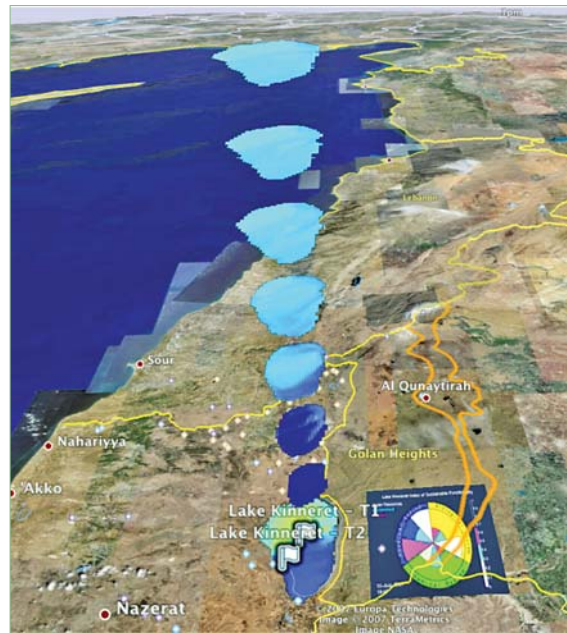
Figure 1. Model output embedded into Google Earth for viewing data from Lake Kinneret (Israel) in the context of the surrounding landscape. Sheets are chlorophyll at 5 m depth intervals from the top to the bottom layer. A colour-coded representation of the measured gradient is used. The schematic adjacent to the lakes is the real time ISF graph.
