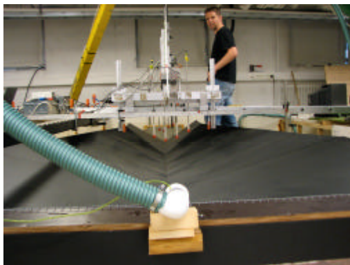
Conductivity probes configured to measure (a) cross-channel and (b) along channel density profiles
