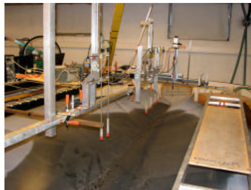
Conductivity probes configured to measure (a) cross-channel and (b) along channel density profiles
